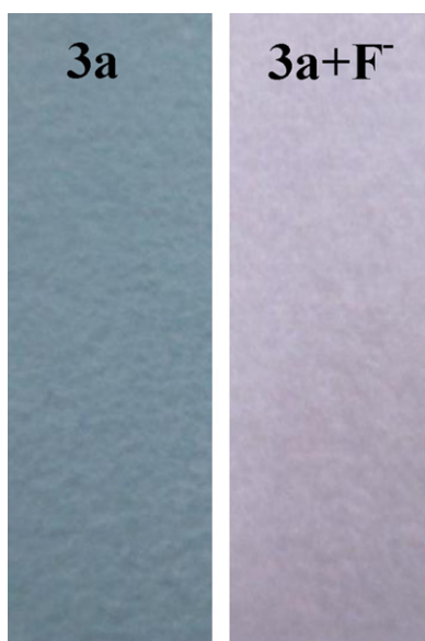
Fig. 7. Observed colour changes of the test-paper of 3a upon detection of F^- in aqueous solution.
